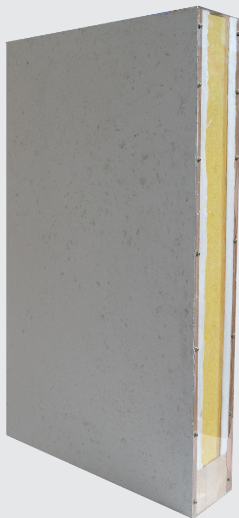
Exterior side lime and hempen mixture Bottom plaster
